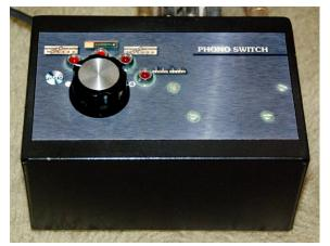
To solve the problem, I constructed the relay-controlled phono switch box shown at left. I didn't want to have to deal with another manual, amp selector switch. The relays are driven from AC adapters at each amp. Those are plugged into the switched AC outlets on the amps. Whichever amp is turned-on gets the connections. Priority logic handles conflicts. A manual override allows amp comparisons.
