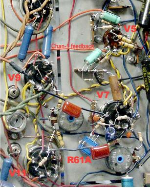
Install the new 1W resistor values: R61 changes from 28.75K to 22K, R63 from 33K to 27K. Note that modern 1W resistors are smaller than the ones found in the unit.
