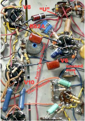
Add the two RC networks R54A/C62A and R60A/C60A. See detail on the previous page. Note the heatshrink at the junction. Since this is sensitive to stray capacitance, do not try to connect the junction to a terminal strip.
