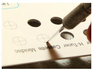
hole, put a gentle, clockwise torque on the blade, while at the same time, applying an outward lateral force. In summary: Simultaneously apply a downward cutting motion, outward pressure and clockwise torque.
