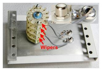
wipers as the lugs which make continuous contact with the inner ring of the wafers. The phono connectors require nylon washers to keep the grounds apart. In the <u>left inset</u>, you can see the nylon shoulder washer needed in front. The nylon flat washer and the supplied ground lug are used in back as seen in the <u>right inset</u>.
