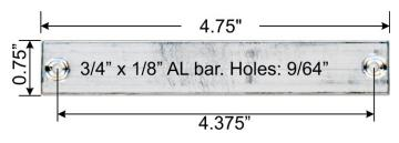
You will need to countersink the holes because the supplied metric screws are not long enough to reliably get purchase through the 1/8" bar stock. (I didn't have longer metric screws and didn't want to spoil the threadings.)
