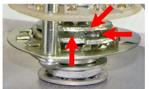
I found that the click-stops were much too stiff, due to the spring being too tight. In the photo at left, the horizontal arrow points out the ball which falls into click-stops. The slanted arrow points to the circular spring and the vertical arrow indicates where you can insert a screw driver to loosen the spring.
