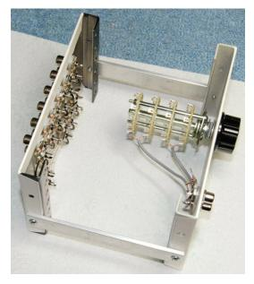
bottom or top cover for this, you will find that they block access to parts of the switch and connectors, making wiring difficult. Without anything to hold the units together, it would be nearly impossible to judge the individual lengths of cable with which to make the connections. These brackets did a great job. Fabrication details are **below**.
