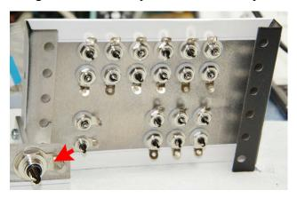
Prewire the rear panel by installing the ground resistors, using a bus structure as <u>at right</u>. The grounds come together at the right Line Out ground lug. The resistor leads soldered to the individual input connectors should not touch the chassis.
