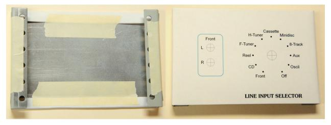
sure that the folds are aligned with the edges as accurately as possible. The paper should be pulled moderately taut but not extremely tight.
