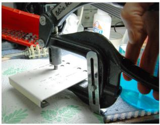
so it's hard to visually align it to the template. To align the punch most accurately with the template, use a sharp point like a scriber to make a hole at the center of the "X" on the template. I recommend using a magnifying visor. Press hard to make it bite into the aluminum, too. Align the template by holding the panel up against the punch center pin and moving it about until the pin slips into the scribed hole. It's quite easy and very accurate.
