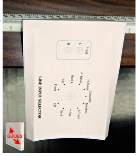
the guides with the edge. Begin by gently pinching the template around the edge, just at the guides. The key to this is gradually sharpening the bend, while adjusting alignment.
