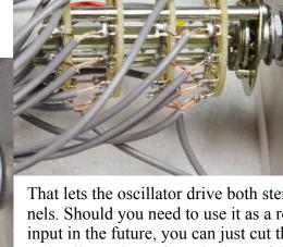
That lets the oscillator drive both stereo channels. Should you need to use it as a regular input in the future, you can just cut the orange and yellow wires. If you look carefully above the yellow wire, you can see the jumper wires for the off-position.
