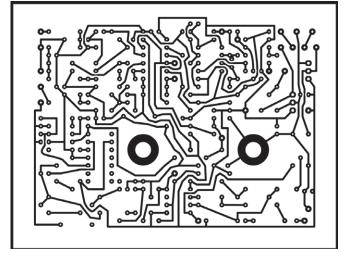
Since there isn't a real silkscreen on the board, some key info is written in the topside metal, including labels for IC's, adjustments, supply voltages and a few external connections. The half-moon shapes indicate the pin-1 end of the IC's. Bottom-side metal is **shown at the bottom of the previous page**.
