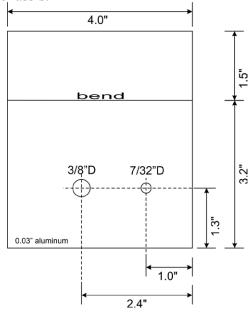
washers, two 1/2" nylon washers and one 3/8" nylon washer. The nylon washers insulate the positive meter terminal from the grounded shield. Press the 3/8" washer into the hole in the shield, so it is even with the metal. The pairs of nuts below the shield are tightened on each other to establish a fixed platform. Notice the nylon washer makes one side lower.
