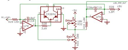
U7B adjusts the current feeding both emitters, to make the collector current of the left transistor track the input signal. So the base-emitter voltage of the left transistor is basically the output value we want.
