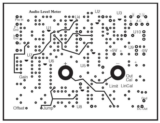
nections, IC's and cap polarities are labeled in magenta. Notice that all IC's are oriented in the same direction. External connection points are illustrated with flea clips, which we used as terminal pins. Orient diodes with their cathode bands as shown.
